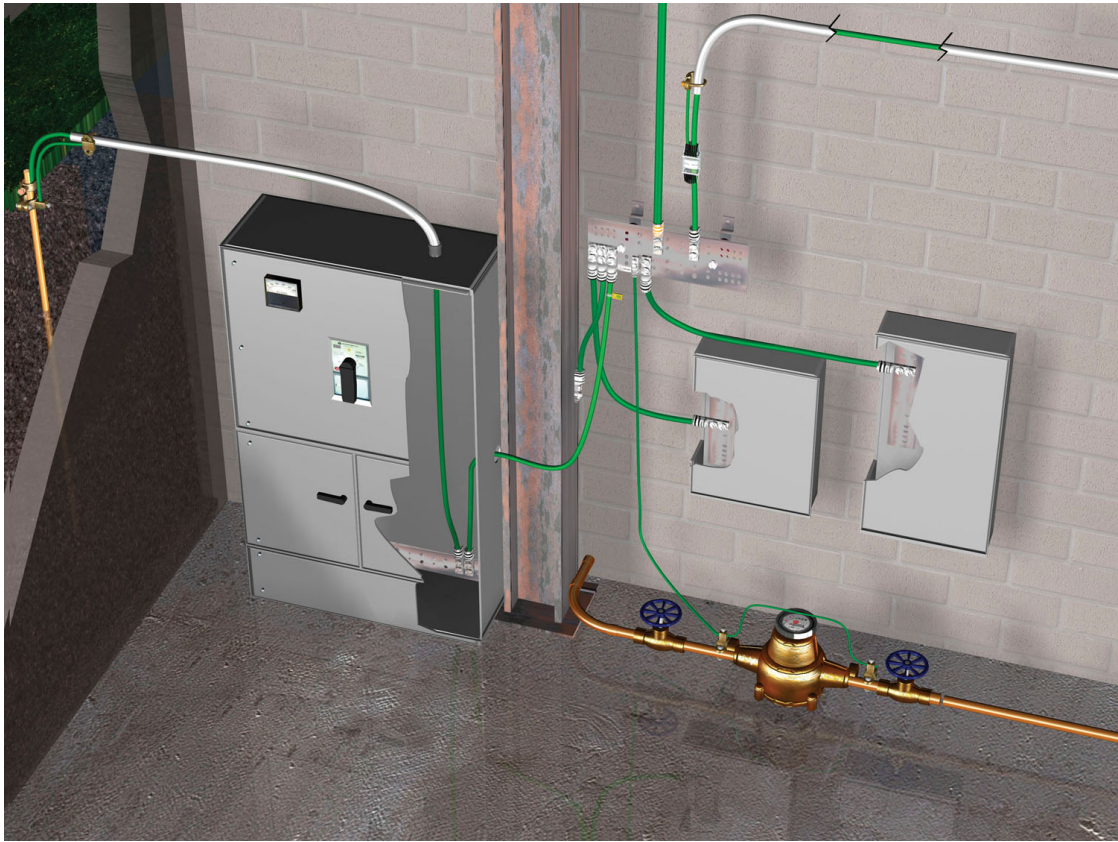
Figure 3: Grounding and Bonding at the Service Entrance
